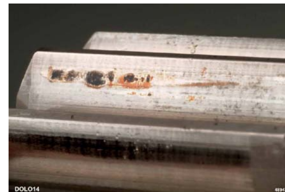
Planet Gear fretting corrosion
